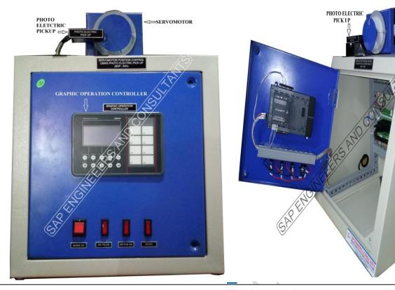
The **SERVOMOTOR POSITION AND SPEED CONTROL TRAINER (SAP – 64A)** gives an idea regarding the construction, operation and application of Servomotor.
